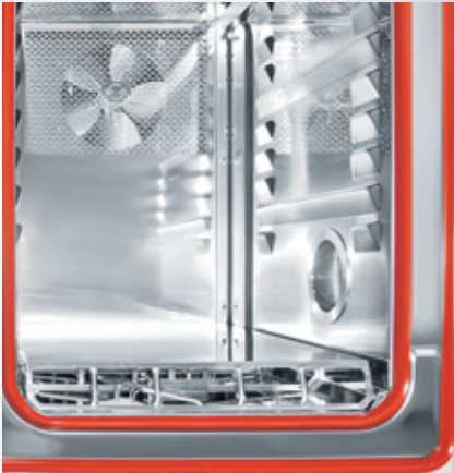
Stainless steel test space
