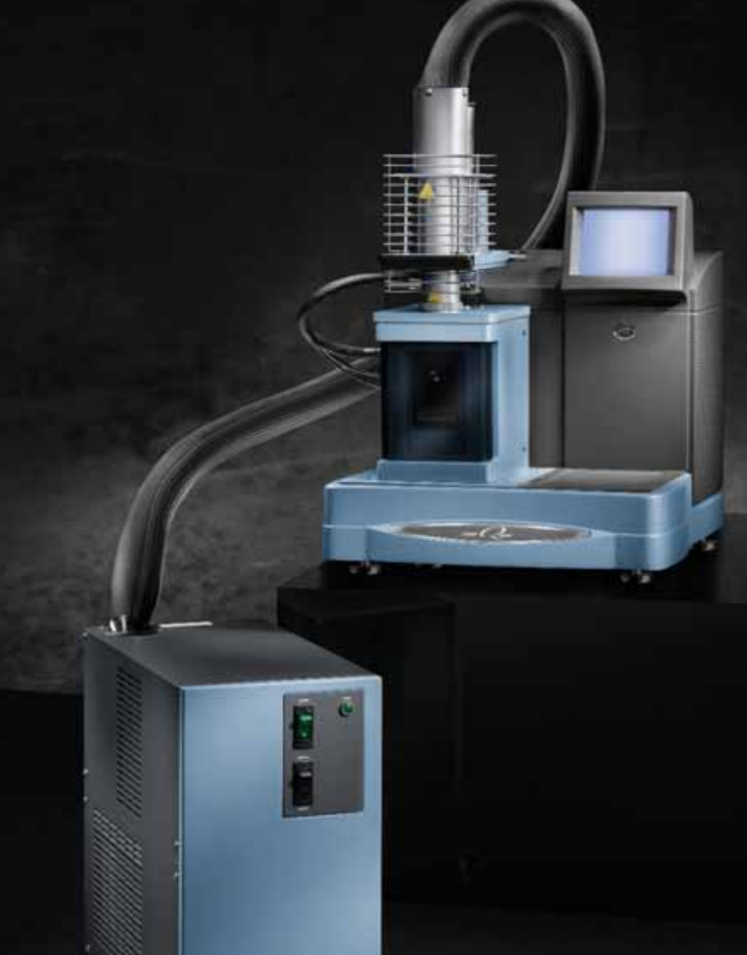
MCA70 Controlled Cooling Rates, from 400°C (upper limit)*
